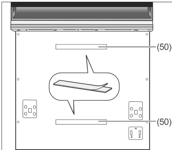
7. With the protective film removed, stick the Velcro straps onto the middle of the recessed areas on the appliance door.
