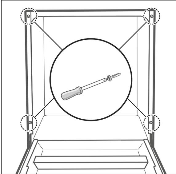
2. Remove the 4 screws from the left and right front edges of the unit.
