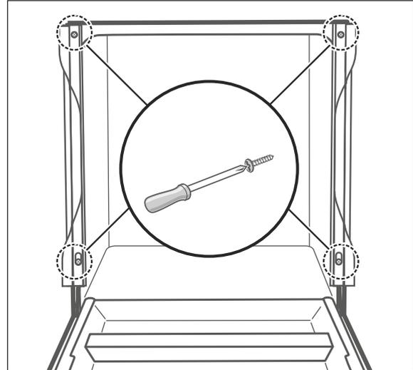
5. Fasten the sound-absorbing strips with the 4 screws.
