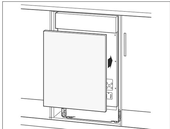
14. Attach the front panel to the appliance door of the dishwasher using the Velcro straps (50), hold the panel in place, and carefully open the appliance door.
