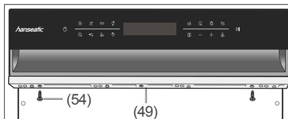
4. If you only need 1 moulding, saw off the 4 protruding feet, clamp the moulding under the control panel and secure it using both countersunk screws (54). Continue with Step 7.
