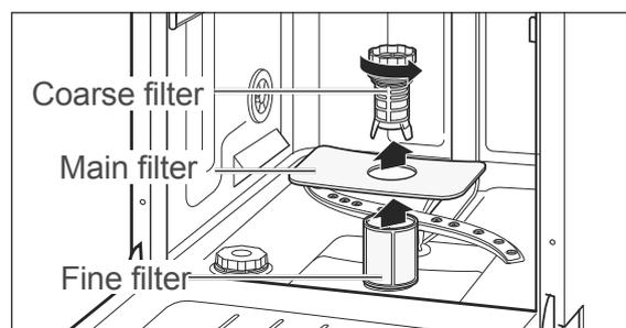
Check the coarse filter, the main filter and the fine filter after each rinse cycle and remove food residues and foreign bodies if necessary:
