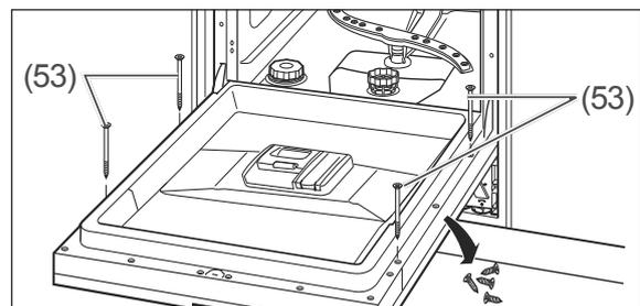
15. Remove the 4 screws from the inside of the appliance door. Screw the front panel in place at these positions using the 4 enclosed screws (53).
