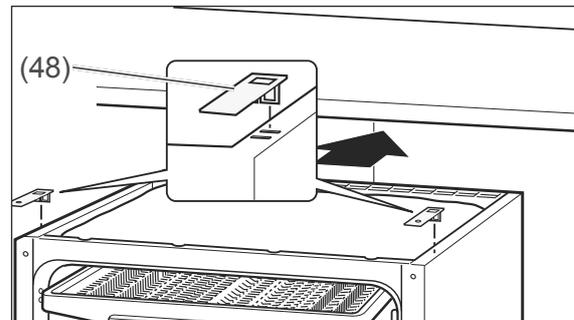
1. Insert the two mounting brackets (48) into the front slots on the top of the appliance so that you can screw the appliance to the worktop later on.
