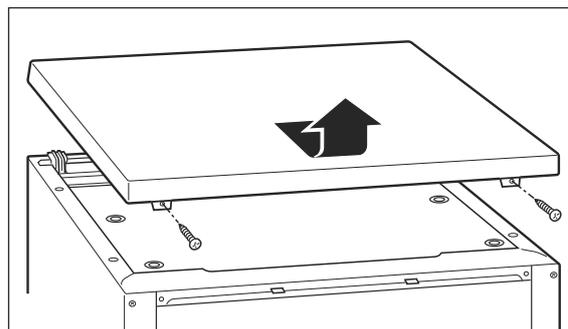
3. Loosen both screws on the reverse side of the covering panel and remove them.
