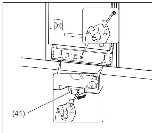
1. Insert a screwdriver into one of the slots and turn the adjustable feet to the height required.
