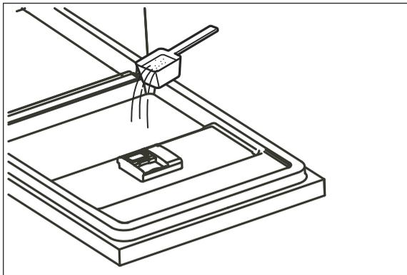
3. Pour the remaining 1/5 of the dishwasher detergent on the inside of the appliance door. Your appliance uses this quantity during the pre-wash programme.
