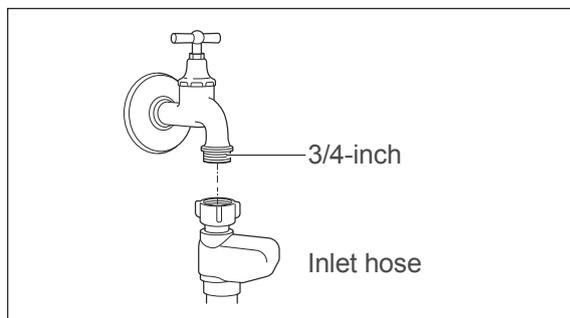
For the water supply, you will need a valve with a 3/4 inch screw connection.
