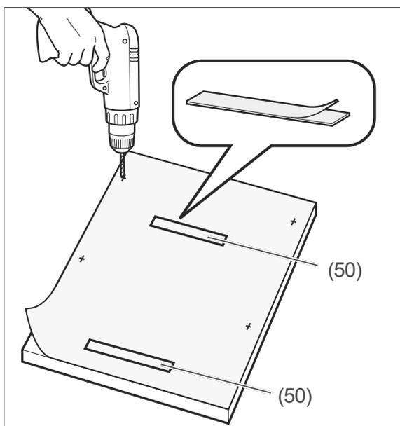
10. Lay the supplied drilling template on the reverse side of the front panel in such a way that the drilling template and the front panel are flush at the top.
