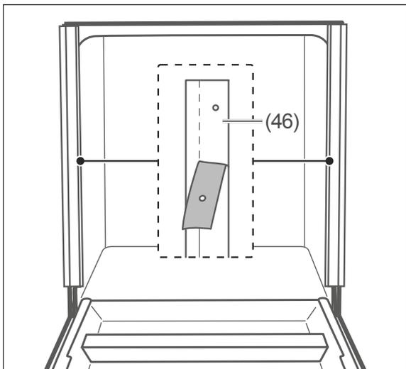
3. Remove the protective films from the sound-absorbing strips (46).
