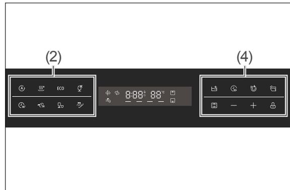
2. Press the respective programme button on the programme selection keypad (2) or on the programme options keypad (4) to select the desired programme. The button will start to light up.
