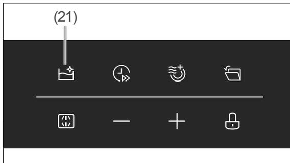
2. Press and hold the
