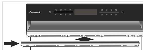
5. If you need more than 1 moulding, turn the lower moulding and push it onto the other mouldings. This hides the feet and makes the surfaces flat.
