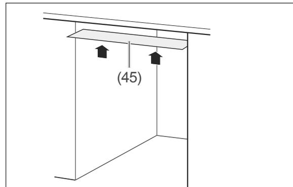
3. Affix the enclosed protective film (45) to the bottom of the worktop. In this way, you will avoid damage to the worktop as a result of hot steam which may be emitted from the dishwasher if the dishwasher door is left open.
