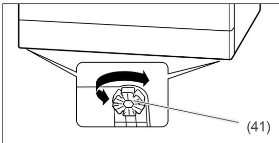
6. In order to compensate for uneven floor surfaces and set up the dishwasher horizontally, you can screw the four adjustable feet (41) in or out. The adjustable feet have slots around their circumference. Insert a screwdriver and turn the adjustable foot.
