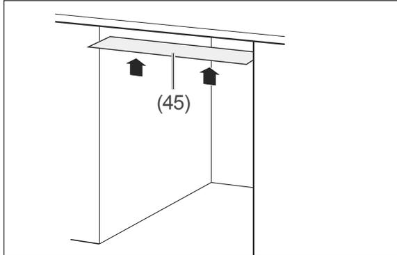
4. Affix the enclosed protective film (45) to the bottom of the worktop. In this way, you will avoid damage to the worktop as a result of hot steam which may be emitted from the dishwasher if the dishwasher door is left open.
