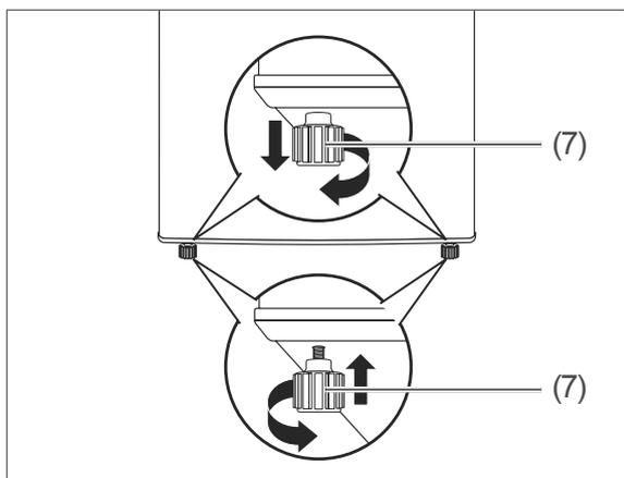
5. Level out any unevenness on the ground using both of the front screw feet (7).
