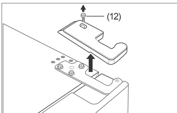
2. Unscrew the screw (12). Then remove the hinge fitting.
