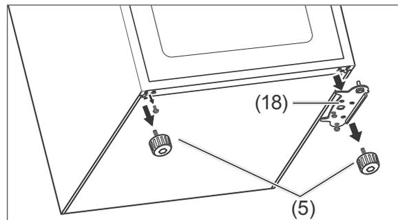
10. Tilt the unit slightly backwards against a wall so that the lower hinge (18) is accessible.
