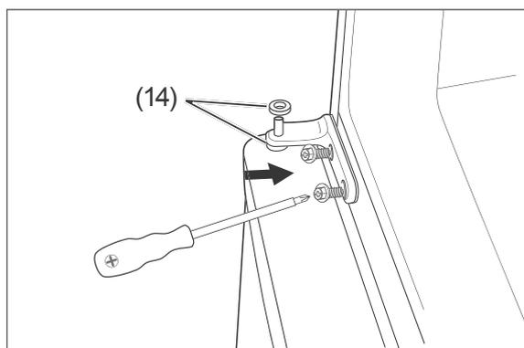
16. Reinsert the middle hinge into the new position. In the process, pay attention to the two plastic discs (14). Screw the hinge tight.
