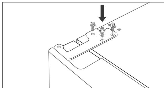
19. Replace the upper hinge and screw it tightly.
