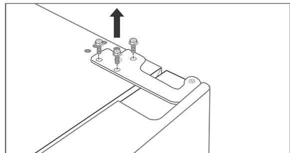
3. Unscrew the 3 screws on the upper hinge and remove the hinge.
