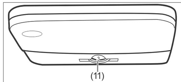
The temperature controller is also (11) used to switch the appliance on and off. It is at the top in the fridge compartment.
