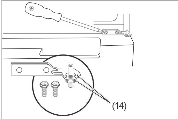
6. Unscrew the middle hinge and remove it. Pay attention to the plastic discs (14). They must later be repositioned correctly in the same place.
