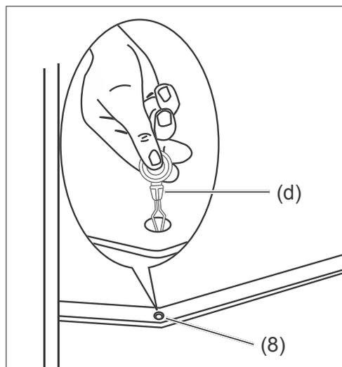
12. The thaw water drain (8) can be found on the reverse side of the refrigerator area above the vegetable drawer. Clean it regularly with the cleaning tool (d).
