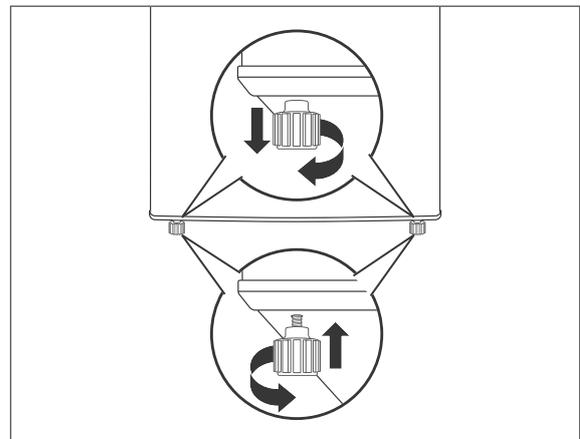
2. Level out any unevenness on the ground using both of the front screw feet.
