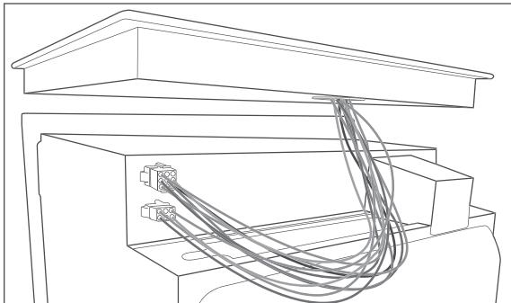
2. Insert the hob plugs into the sockets on the top of the cooker. Do not use any force. The plugs are coded. Polarity reversal is therefore not possible.
