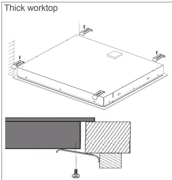
6. Depending on the worktop's thickness, attach the 4 brackets by screwing them to the hob from below. This will prevent the hob from moving.
