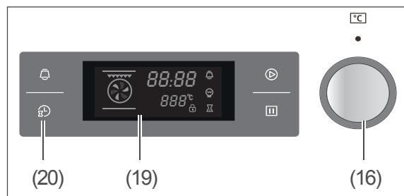
1. Tap the sensor (20). The indicator showing the current hour will flash.
