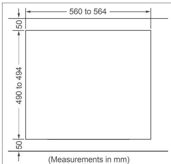
1. Use a jigsaw to cut a hole in the worktop for the hob. It must have the following dimensions.
