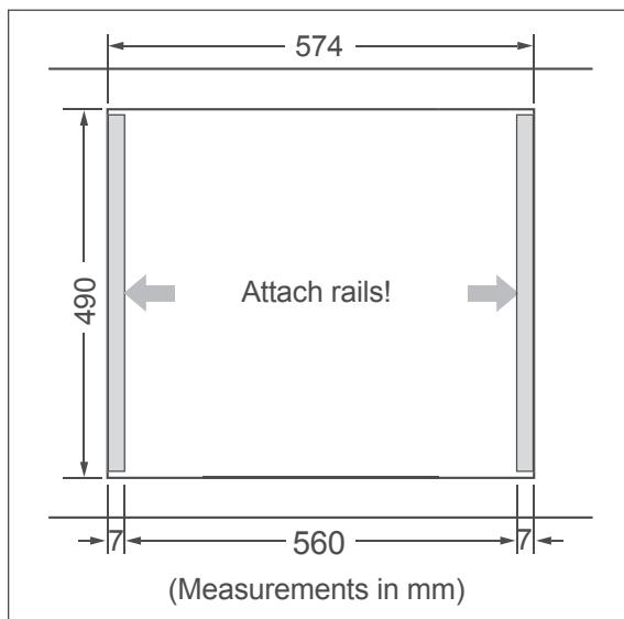
2. If a hob was already installed, the cut-out section must be no larger than:
