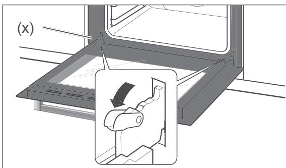
2. Fold the brackets (x) on both sides all the way forward. Use a screwdriver if necessary.
