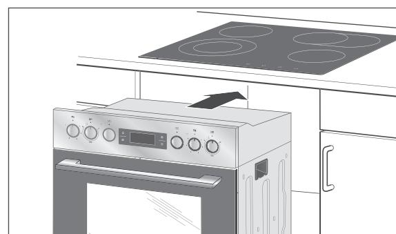
1. Use the carrying handles on the side of the oven to lift it and then push it as far back into the built-in cabinet so that the connections and earthing screw for the hob can still be easily reached.
