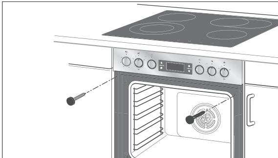
5. Screw the oven to the built-in cabinet with the two screws which have been supplied.
