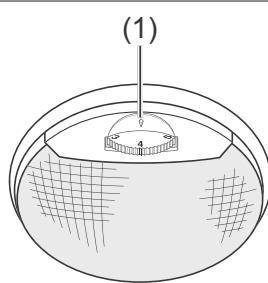
The temperature controller (1) is also used to switch the appliance on and off. It can be found at the top of the fridge compartment.
