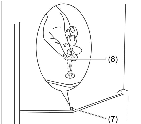
11. The thaw water drain (7) can be found on the reverse side of the refrigerator area above the vegetable drawer. The cleaning tool (8) can be found in the opening to the thaw water drain. Use it to clean the thaw water drain.
