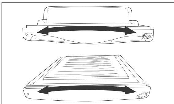
17. Unscrew the hinge bushings from the top of the fridge compartment door and on the bottom of the freezer compartment door and screw them back on tightly on the opposite side.
