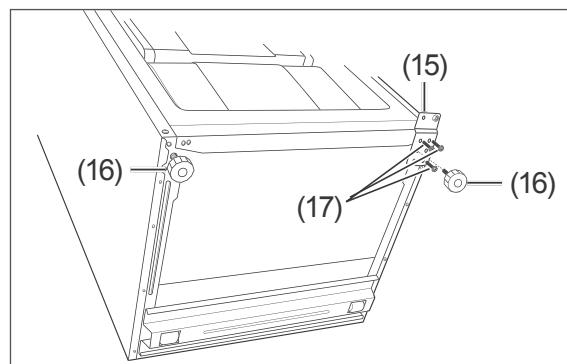
8. Tip the appliance back as far as possible (45° max.) in such a way that the front feet of the appliance (16) and the lower hinge plate (15) are easy to reach.
