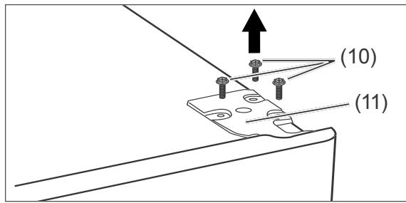
3. Loosen and remove the screws (10) and remove the upper hinge plate (11).
