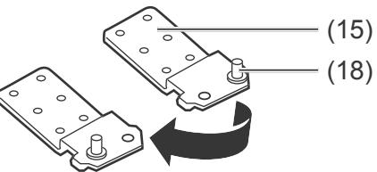
12. Replace the hinge bolt (18) as shown above.
