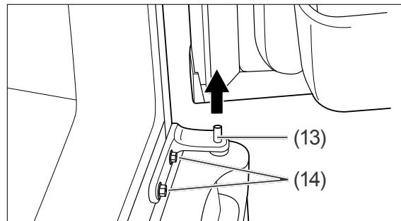
5. Open the fridge compartment door and lift it vertically upwards from the bolt on the middle hinge (13). Set the door aside.
