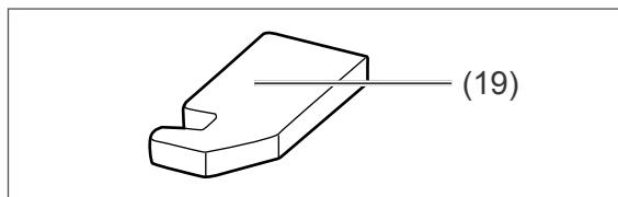
24. Press the hinge faceplate (19) onto the hinge plate and the covering plate into the holes on the opposite side. This is the final step in changing the direction in which the door closes.
