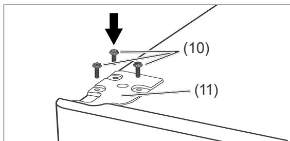
22. Place the upper hinge plate (11) on the fridge compartment door and then screw it tight using the three star-headed screws (10).
