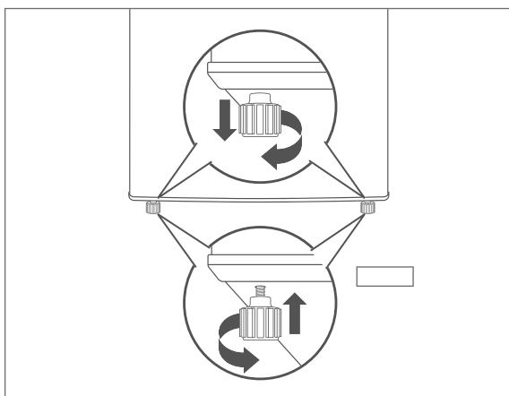
3. Level out any unevenness on the ground using both of the front screw feet.
