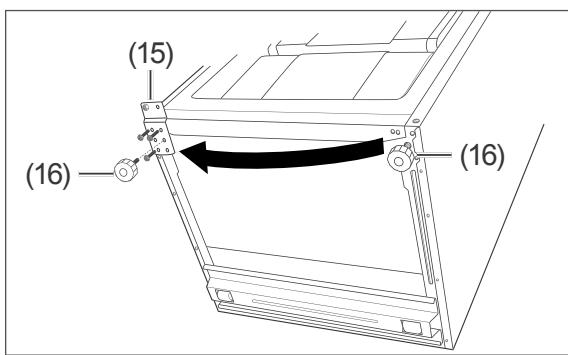
13. Screw the hinge plate back onto (15) the opposite side.
