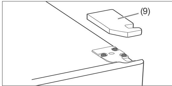
2. Carefully lift the hinge faceplate (9) up with the help of a flat-headed screwdriver. Also remove the covering plate on the opposite side.
