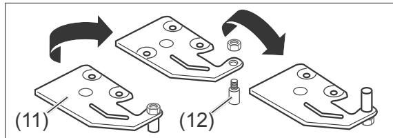
4. Unscrew the nuts from the hinge bolts using a size 10 spanner. Unscrew the hinge bolts (12) from the upper side of the hinge faceplate (11) and rescrew them back onto the bottom. Rescrew the nuts tightly on to the hinge bolts.
