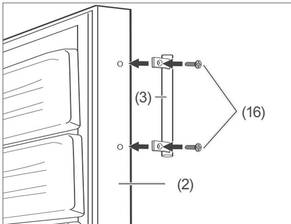
2. Screw the door handle (3) to the appliance door (2) using the screws (16) provided.
