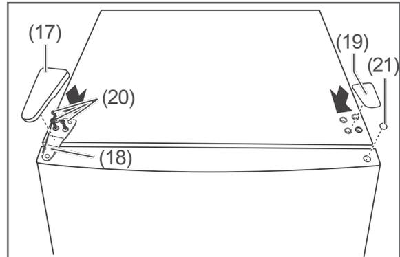
1. Tighten the upper hinge (18) with the screws (20).
