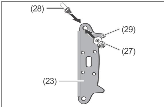
5. Turn the lower hinge (23) over and screw the hinge pin (28) and snap ring (29) back on.
