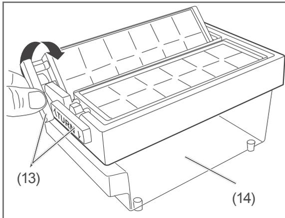
2. To remove ice cubes, turn the levers (13) clockwise.
