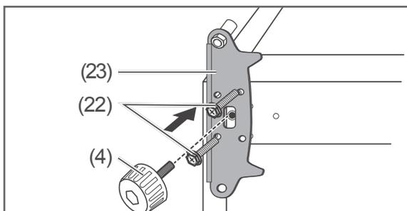
1. Screw on the lower hinge (23) on the left with the two screws (22) and screw the screw foot (4) back in.
