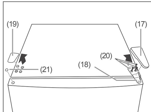
1. Remove the hinge cover (17) of the upper hinge (18) and the opposite cover (19).
