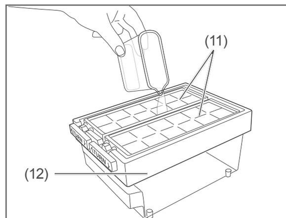
1. Fill the ice cube moulds (11) of the ice cube maker (12) that comes supplied to approx.  $\frac{3}{4}$  full with fresh drinking water and place it horizontally in the freezer. It is best to use a filling container for this (not included in the package contents).
