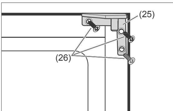
7. Unscrew the three screws (26) on the upper hinge (25) and remove it.
