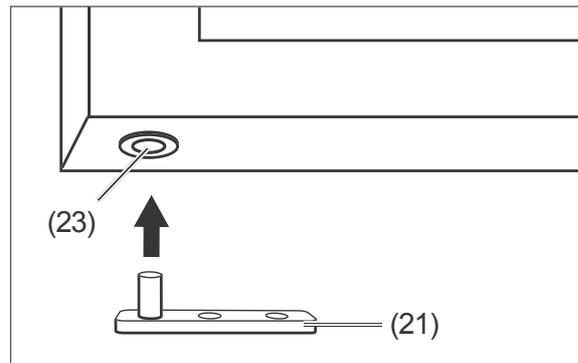
5. Rotate the glass door 180° and place the hinge plate (21) into the plastic insert (23).
