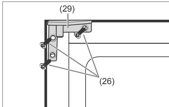
10. Mount the included upper hinge for changing door hinge (29) on the upper left side using the screws (26).
