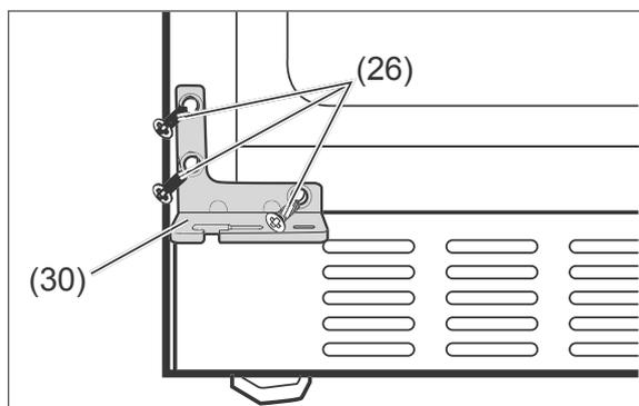
11. Mount the included lower hinge for changing door hinge (30) on the lower left side using the screws (26).
