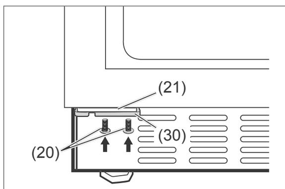
13. Screw the hinge plate (21) onto the lower hinge (30) with the screws (20).
