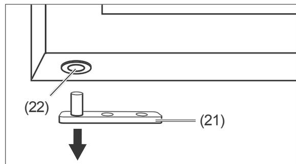
4. Remove the hinge plate (21) from the plastic insert (22) on the lower edge of the glass door.
