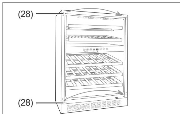
9. Remove the three dummy plugs (28) from the threaded holes above and below and move them to the opposite side.
