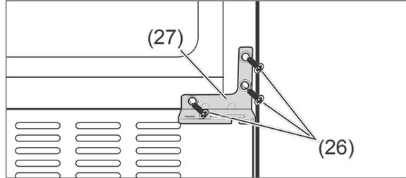
8. Unscrew the three screws (26) on the lower hinge (27) and remove it.
