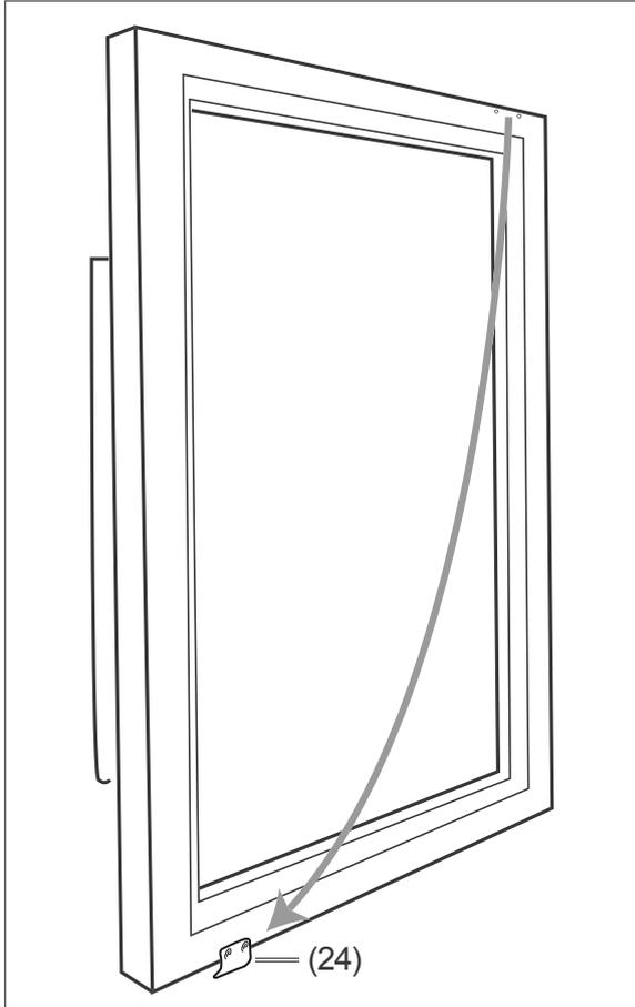
6. Unscrew the metal plate for the light switch (24) from the door frame and screw it on the door frame of the opposite side (there are 2 small holes reserved). Pay attention to the direction when screwing the metal plate. Set the glass door aside.
