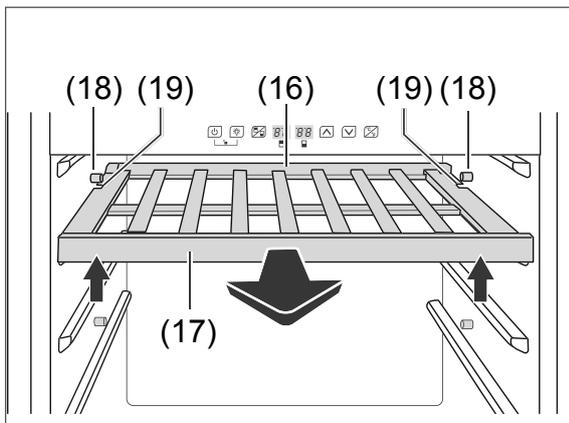
In doing so make sure that the spacers (18) slide into the guide rails (19).
