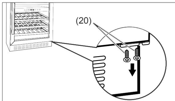
2. Unscrew both screws (20) beneath the lower hinge.
