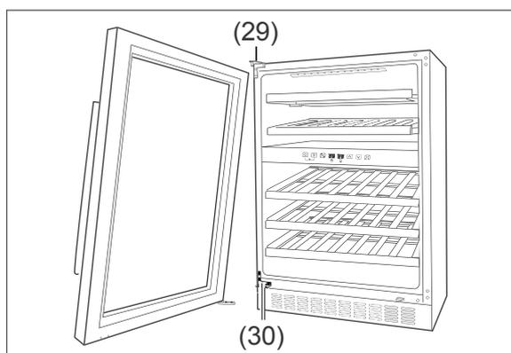
12. First insert the glass door into the upper hinge (29) then onto the lower hinge (30).
