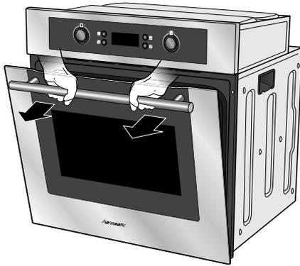
4. Pull the door slightly towards you and then guide it forwards out of its hinges from below.
