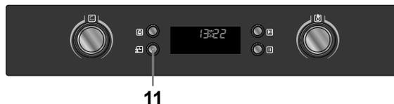
7. Press the 11 button again. The two dots between the two display blocks will start to flash; the time has now been set.
