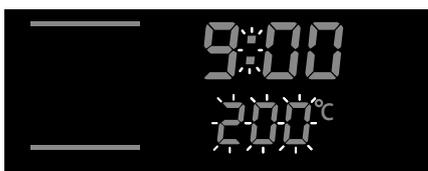
The time indicator 9:00 will appear; the temperature indicator (here: 200 °C) and the two dots between the hour and minute display will start to flash.
