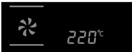
The heat is produced by top/bottom heat and is distributed evenly by the fan.
