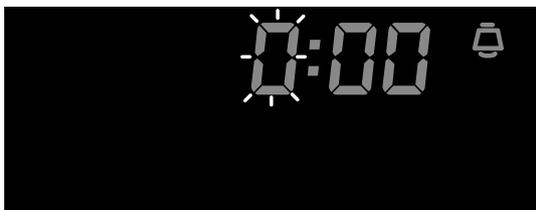
The time indicator will appear on the display with its first 0 flashing, as well as the bell symbol at the top right edge.
