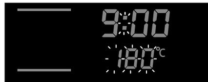
The time indicator **9:00** will appear; the temperature indicator (here: 180 °C) and the two dots between the hour and minute display will start to flash.
