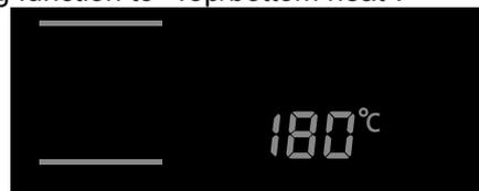
5. If necessary, use the right toggle switch 15 to adjust the temperature. **Notice:** You can adjust the temperature in sequences of 5 °C.
