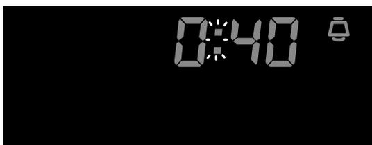
The time has now been set; the two dots between the hour and minute display will flash.
